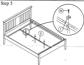
Fix in support leg with bolt 'M'.
