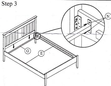
Put in cross bars and fix in bolt 'N' as shown in diagram and tighten all bolts.
