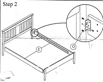
Hook the side rail to bolt as shown and don't tighten the bolt yet.
