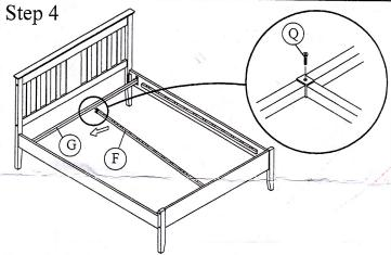
Fix center bar 'F' to cross bar 'G' by follow like diagram as shown.
